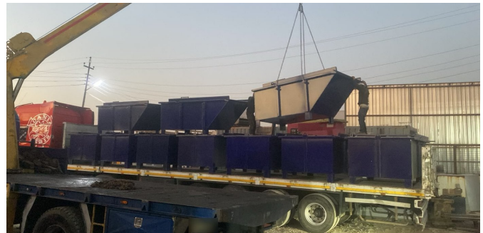
Fabricated steel dumpsters loaded for delivery
